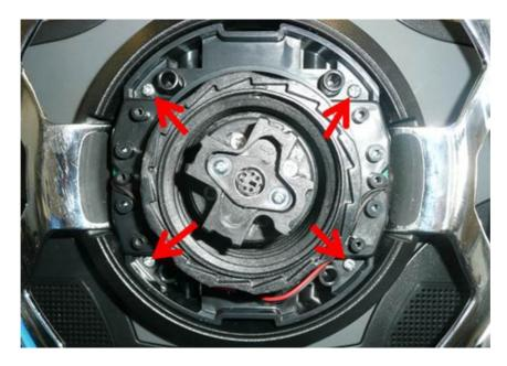
5. Remove the piece holding the gear paddles (be careful not to break the wires)
